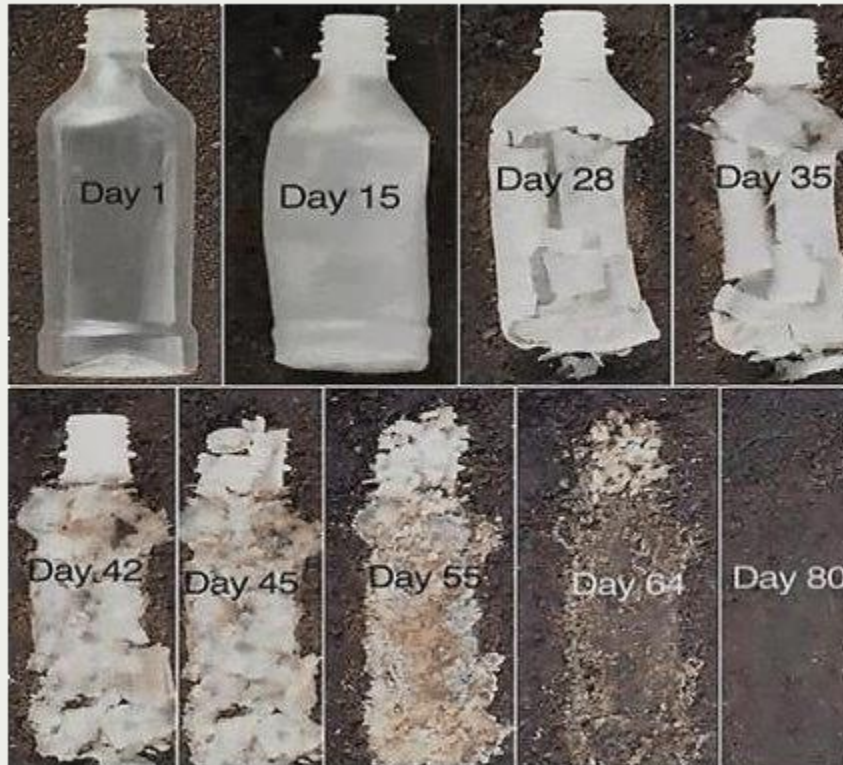
PHA bottle biodegradation, type Biopol™, by incubation in mud for 80 days (Sudesh et al., 2000)
